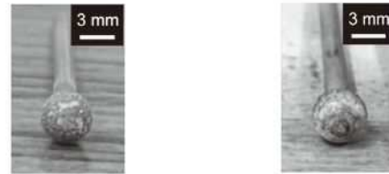
(a) Pure water (b) Saline Fig. 8 \text{TiO}_2 deposited tool surface
